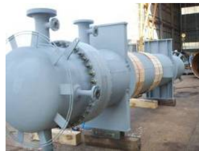
H/Ex for HDO Revamping Project
